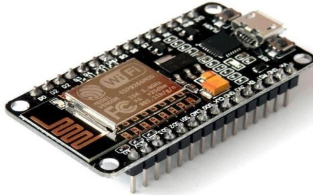
Fig 2: Node MCU -ESP8266
